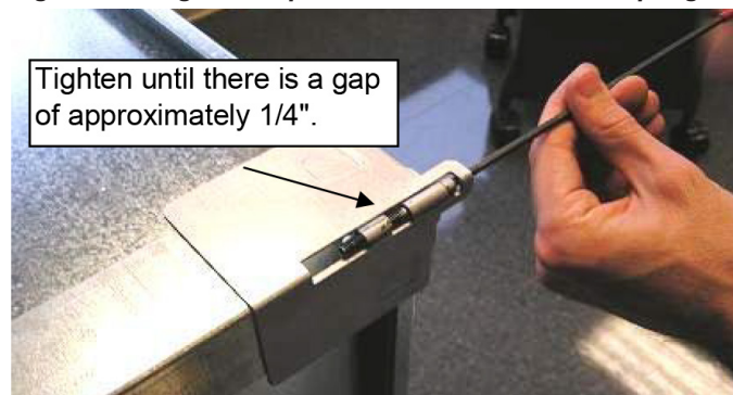
Figure 115: Tighten Cap Screw to 1/4 in. of the Coupling
